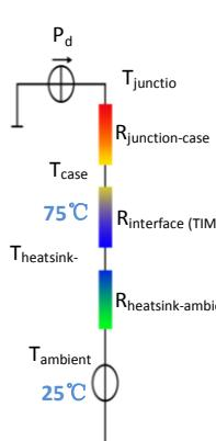
\*Thermal resistance is a heat property and a measurement of a temperature difference by which an object or material resists a heat flow.
