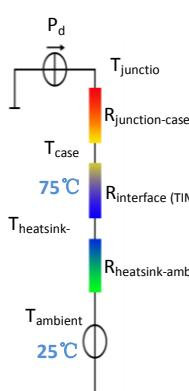
\*Thermal resistance is a heat property and a measurement of a temperature difference by which an object or material resists a heat flow.
