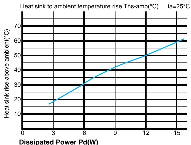
\* Please be aware the dissipated power Pd is not the same as the electrical power Pe of a LED module.
