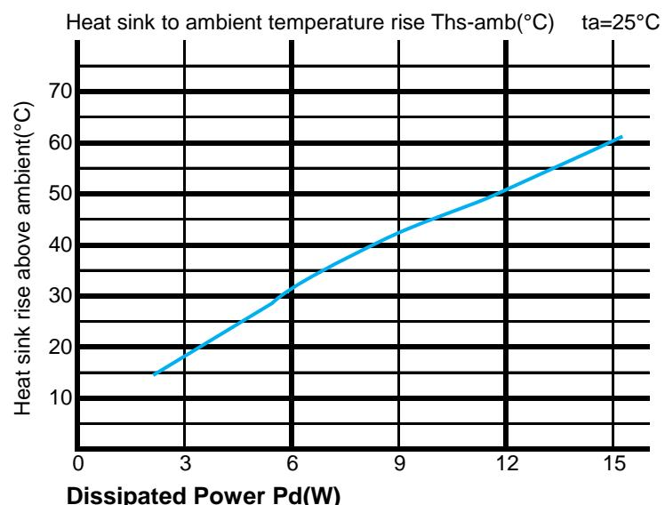
\* Please be aware the dissipated power Pd is not the same as the electrical power Pe of a LED module.
