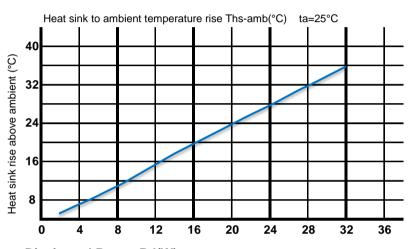
**Dissipated Power Pd(W)**
