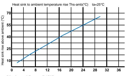
**Dissipated Power Pd(W)**
